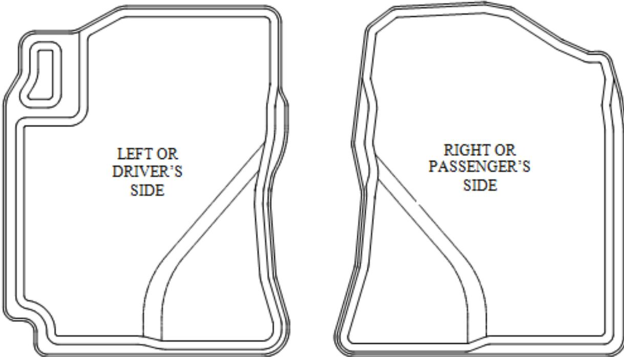
**NOTE TO COROLLA OWNERS:** IF YOUR COROLLA DOES NOT HAVE THE FACTORY ALL-WEATHER GUARD PACKAGE WHICH INCLUDES HEATER DUCTS UNDER THE FRONT SEATS, THIS LINER WILL NOT FIT YOUR VEHICLE CORRECTLY. YOU CAN TELL IF YOU HAVE THE HEATER DUCTS BY THE LARGE RAISED AREAS IN THE FRONT FLOOR PANS LOCATED ALONG THE TRANSMISSION TUNNEL EXTENDING AT AN ANGLE ACROSS THE FLOOR PANS. ATTACHED ON THE BACK OF THIS PAGE ARE PHOTOS OF THESE RAISED AREAS.
