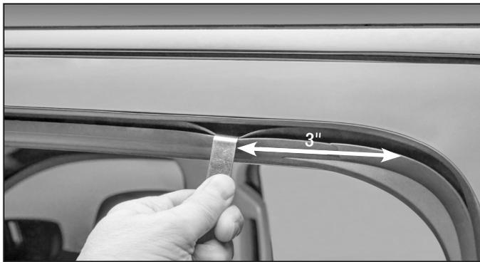
**1** Make sure that the window is clean and dry. Then, pull down the 2nd weather-strip with the provided tool approximately 3" from the rear edge. *Asegúrese de que la ventanilla esté limpia y seca. Luego tire del burlete hacia abajo con la herramienta provista, aproximadamente 3 pulgadas del borde trasero.*
